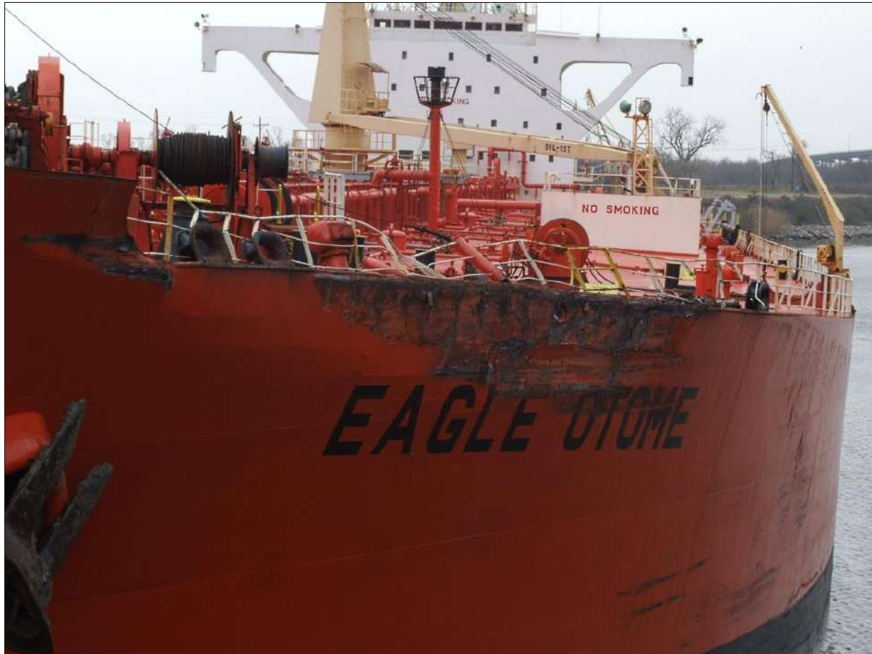
Figure 10. Portside damage to the Eagle Otome .
