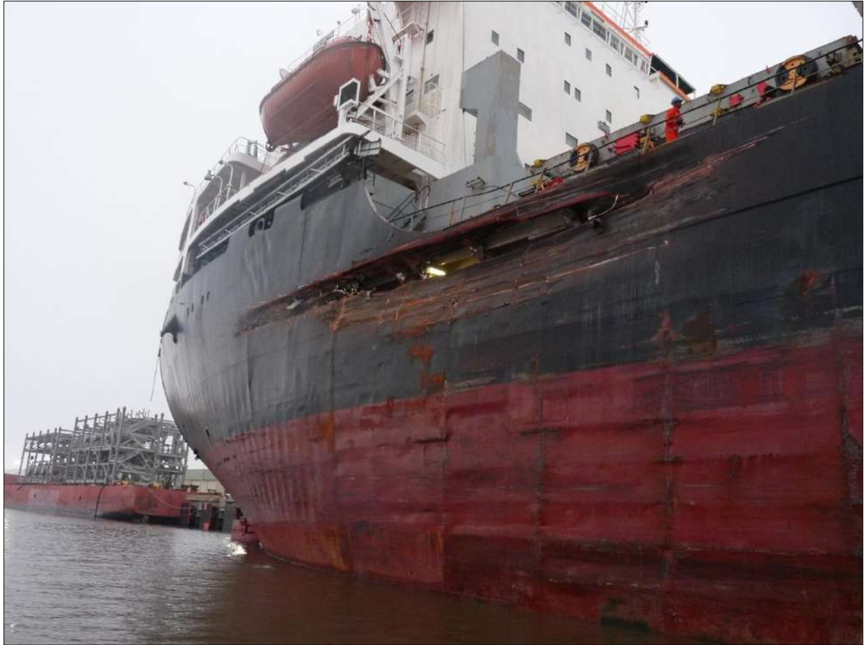
Figure 12. Damage to the Gull Arrow .
